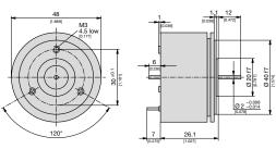
Fig. 2. KINAX 3W2 with special drive shaft at front and at rear. At front: Ø 2 mm [0.078"], length 12 mm [0.472"]. At rear: Ø 2 mm [0.078"], length 6 mm [0.236"].
