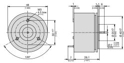
Fig. 1. KINAX 3W2 with standard drive shaft at front only, Ø 2 mm [0.078"], length 6 mm [0.236"].
