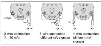
Fig 9. Electrical connection via screw terminals. Only for NEX and ATEX version.
