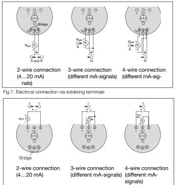
Fig 8. Electrical connection via pads. Only for NEX version.
