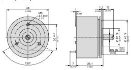
Fig. 3. KINAX 3W2 with special drive shaft at front only, Ø 6 mm [0.236"], length 12 mm [0.472"].
